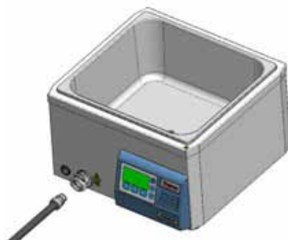
Figure 3-3– GP Bath Drain Hose
